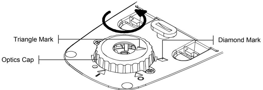
2. Install UV filter optics cap by aligning triangle in cap with the diamond in the bottom housing. Rotate optics cap clockwise until the triangle on the cap meets the triangle/circle on the bottom housing.
