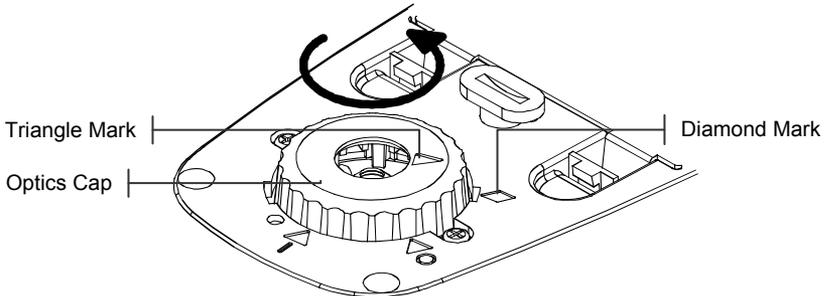
3. Carefully remove the optics cap by lifting upwards and set aside.
