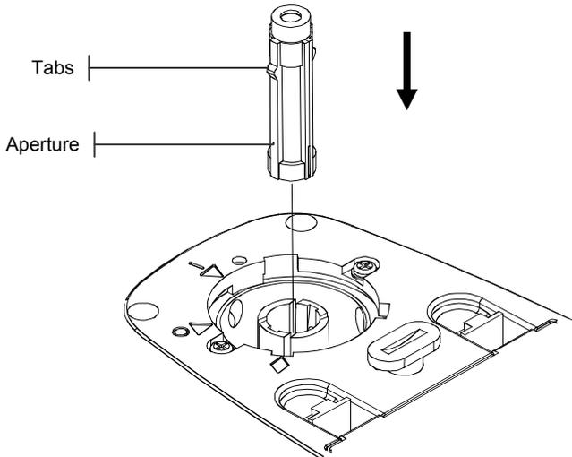
8. Slide aperture into opening. Finish pressing aperture into position using the other end of the extraction tool. A click is heard when the aperture is properly seated.
