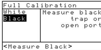
10. *To measure open port (no trap)*, unlatch the shoe and point the instrument towards a dark area that is shielded from light (such as under a table or desk). Press the read switch (located in front of the optics) with your finger. Make sure your finger does not cross the light path during the measurement.
