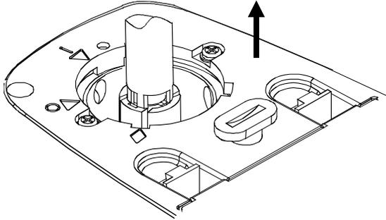
6. Carefully lift aperture tool upward. The old aperture will be attached to the tool fingers. Remove old aperture from tool and set aside.
