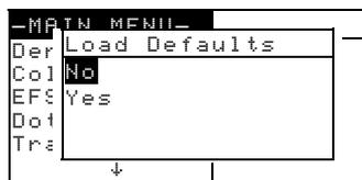
2. Use the Tab Down key ↓ to highlight Yes. Selecting No returns the instrument to normal operation without restoring defaults.
