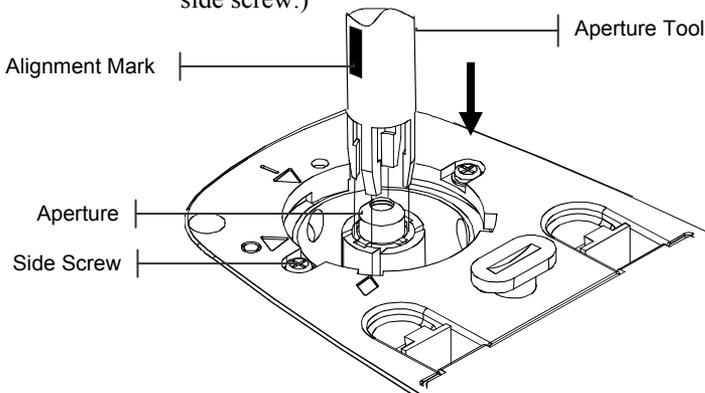
5. Press the tool down (approx. 12mm) on the aperture with slight pressure. A low, click is heard when properly seated.
