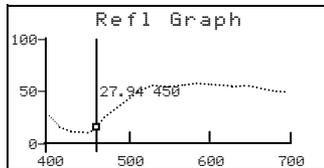
2. Use the Tab Up key ↑ or Tab Down key ↓ to view the data in 10nm increments, along the reflectance curve.
